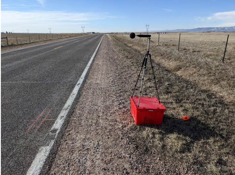
Figure 1 Sound Level Meter Setup and Pass by Distance Marked by Red Chalk on the Road
