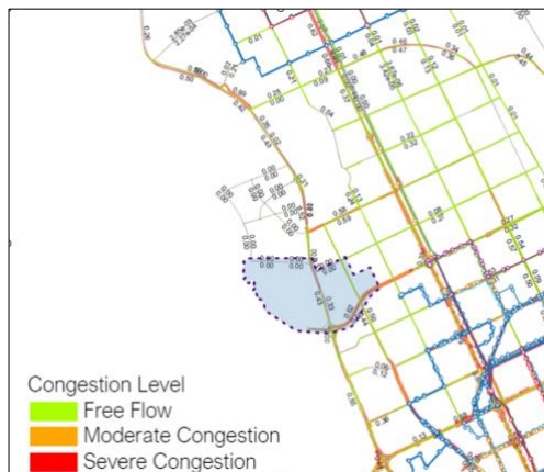
Figure 15. Level of service on roadways without the New Murabba project (Reference scenario). Congestion is represented as volume to capacity ratio: Free Flow (0 to 0.7), Moderate (0.7 to 1) and Severe (>1)
