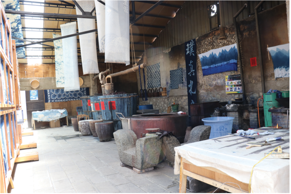
Figure 23. Indigo dye vats and other equipment within the Puezhen Tie-Dye workshop. Zhoucheng, Dali City, Dali Bai Autonomous Prefecture, Yunnan. May 26, 2019. Photograph by Jon Kay.
