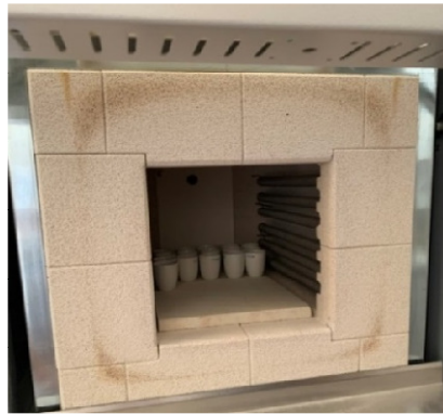
Figure 6. Burning samples in ash oven for ICP-OES analyses
