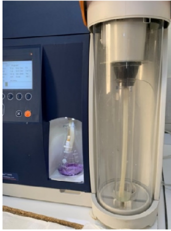
Figure 5. Determination of the total amount of nitrogen in the Kjeldahl device
