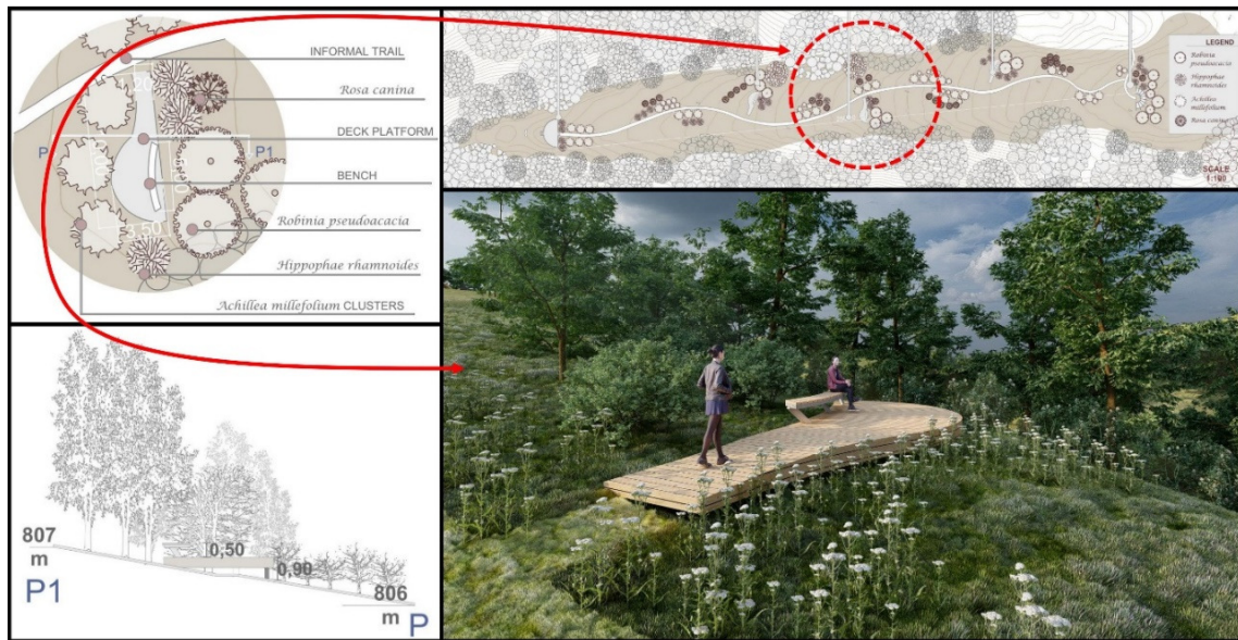
Figure 11. Conceptual design for 'Resting Spot': informal trail, deck platform, and R. pseudoacacia and other species planted
