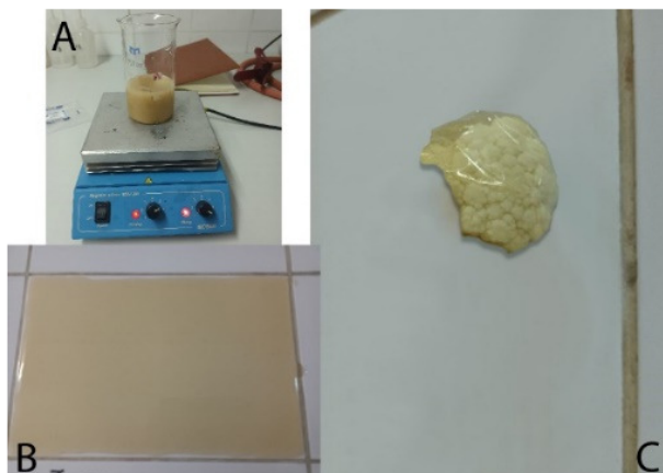
Figure 1. Preparation and application of chitosan film. A) Formation of chitosan film. B) Dried chitosan film ready for use. C) Cauliflower florets wrapped in chitosan film for bio-preservation studies
