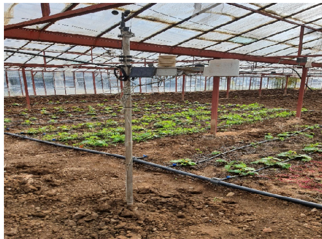
Figure 2. Climate station placed on the field for a Et-based irrigation program
