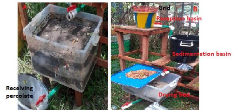
Figure 2: Treated sludge (biosolids) in drying bed (A), Sludge treatment platform with adapted unplanted drying bed (B)
