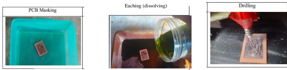
Figure 2. The stages of PCB making process
