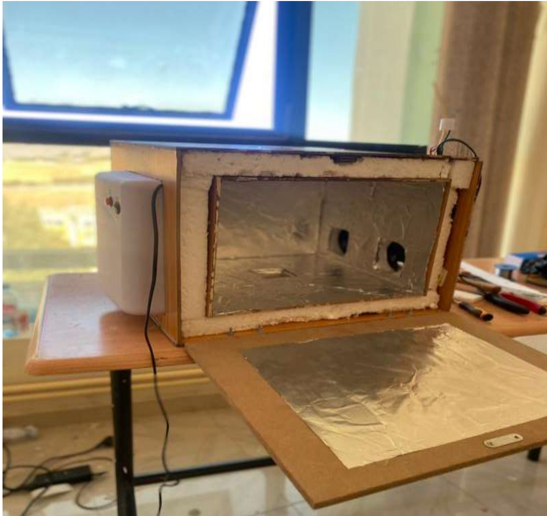
Figure 1: The drying chamber of Indirect Smart Solar Dryer (ISSD) in the laboratory 5-2. Operational evaluation of the dryer (SISD)
