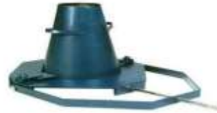
Fig 4.2: Slump Test in progress
