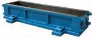
FIG 4.1: Moulds used for testing concrete
