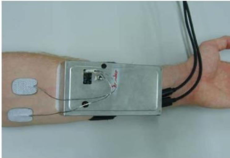
Fig. 1. Coupler unit attached to the lower arm using fixed gel electrodes.
