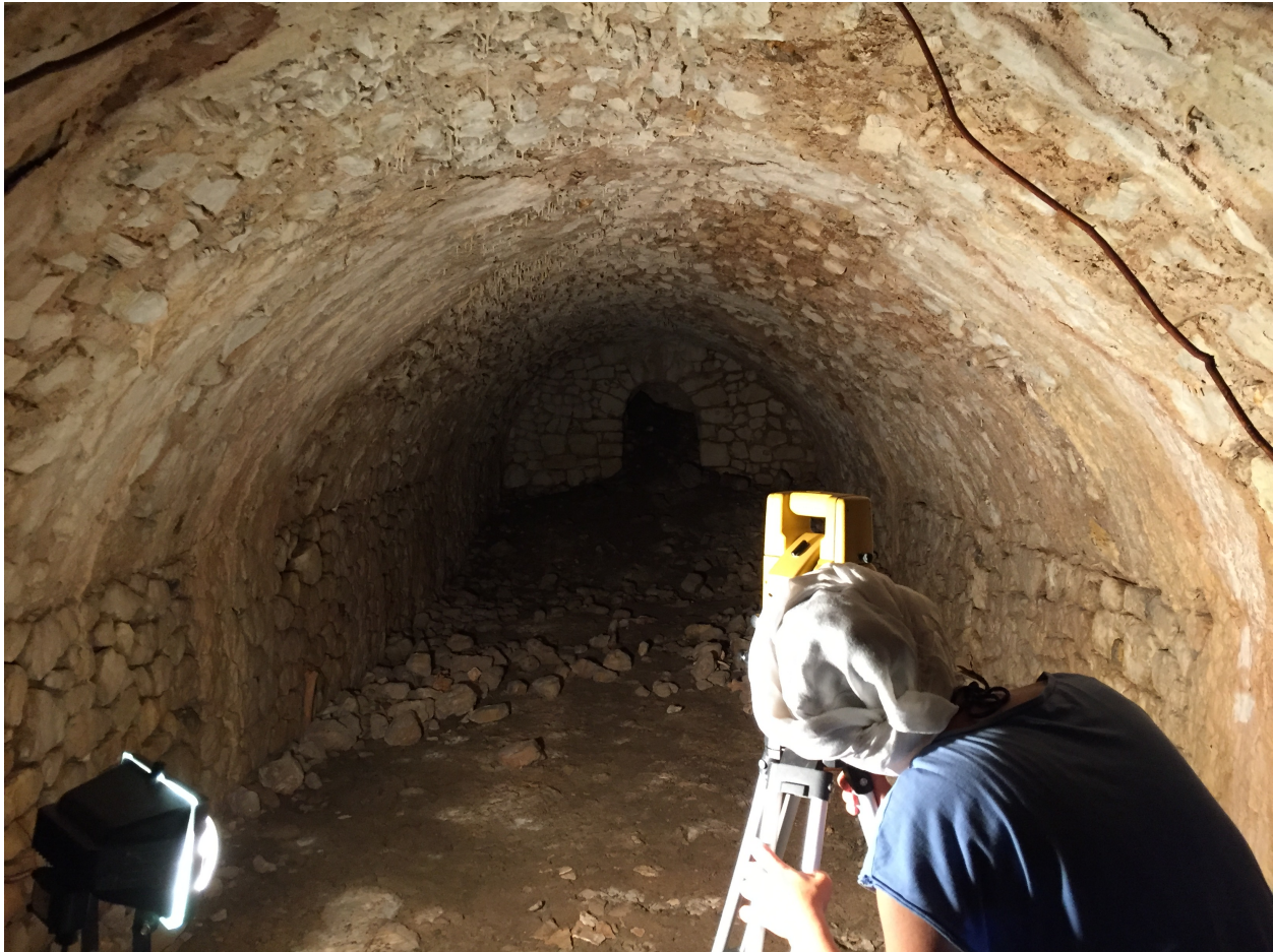
Figure 3. Recording of ground control points with a total station in the eastern cryptoporticus in 2016.
