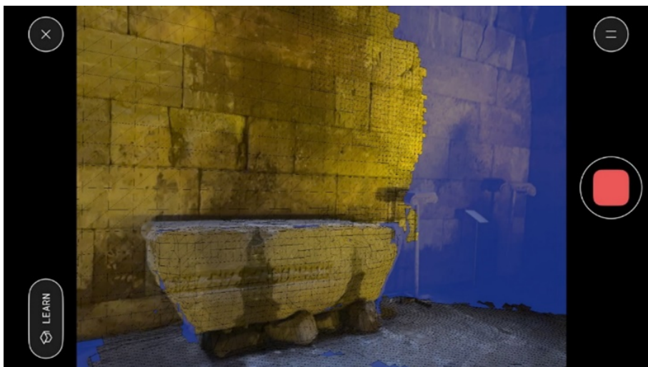
Figure 6. Scanning Process with Polycam Pro Software (Polycam Software. Available online: https://poly.cam/ , paid subscription start: 22.01.2024).
