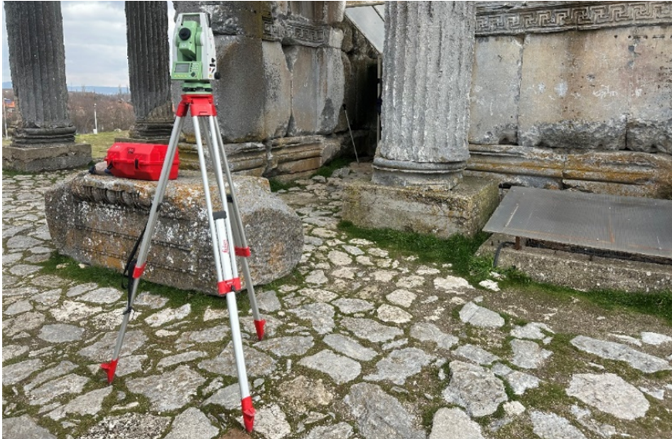
Figure 3. Total Station Laser Measurement and Point Transfer to the Lower Gallery Session Operations.
