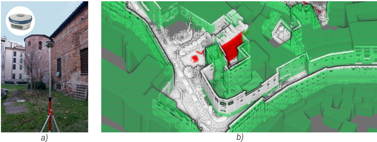
Figure 8. GNSS data acquisition: a) GNSS receiver during the 20 minutes data acquisition phase in front of the roman towers, in the Archaeological Museum backyard; b) 3D scans georeferenced through the GNSS data.
