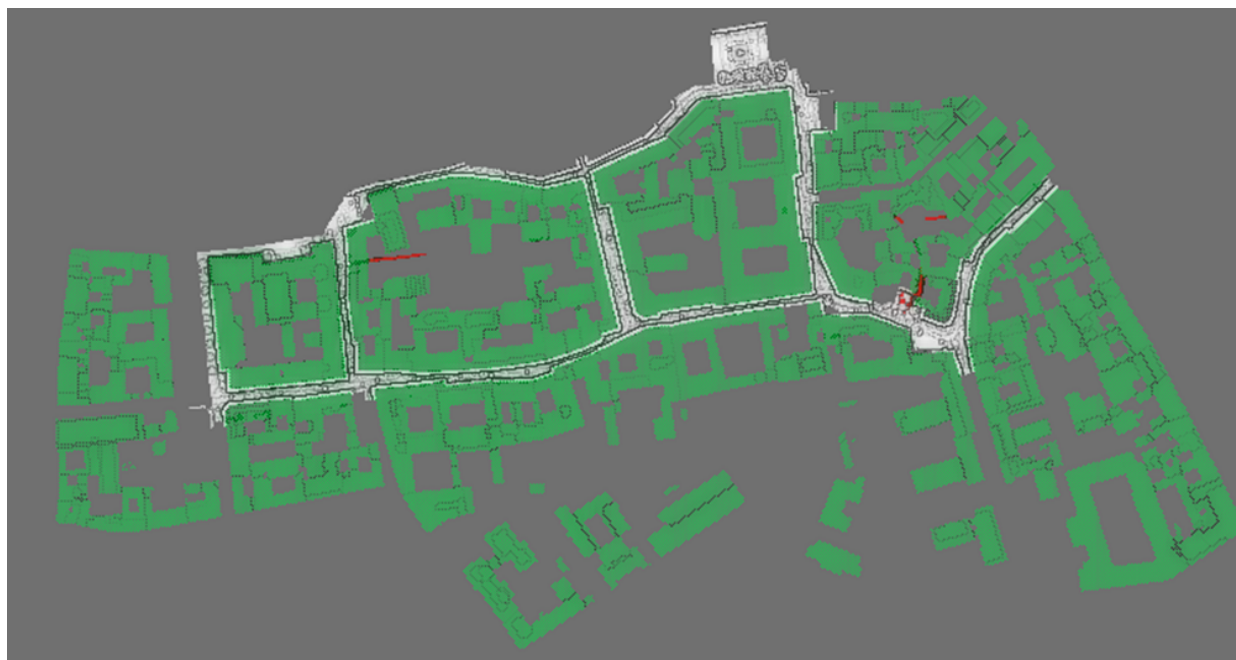
Figure 10. Integration between the mobile lidar data with the terrestrial laser scans mutually aligned with ICP and georeferenced using differential GNSS. Such data, here represented in gray, are overlaid on the city's provided georeferenced plan (green). The figure also illustrates the path traversed by the mobile lidar operator while scanning the outdoor areas (red).
