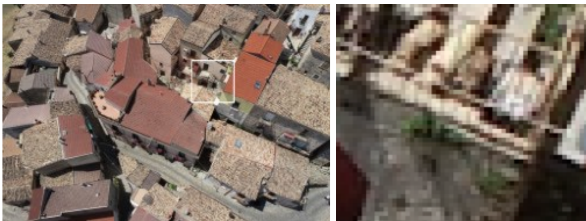
Figure 5: Image quality of the pictures from mini UAVs (DJI mavic mini 2. Image resolution: Ground Sample Distance (GSD) = 2 cm/pix. (picture by authors).
