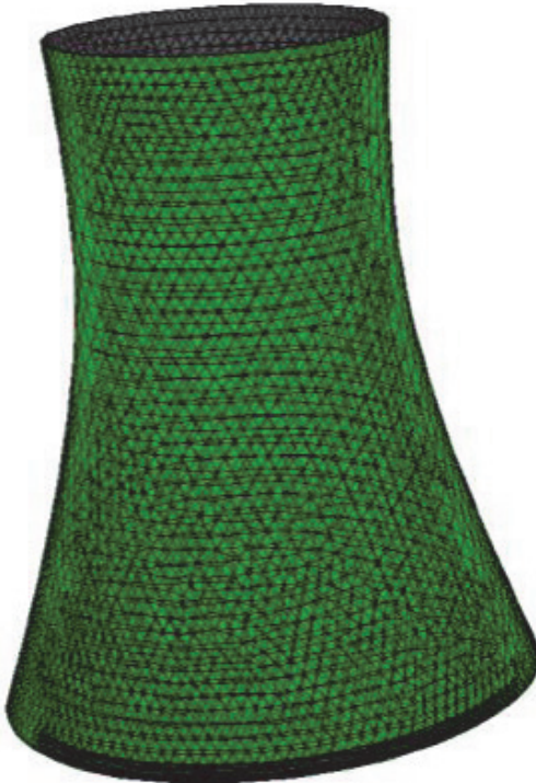
(a) The cooling tower mesh
