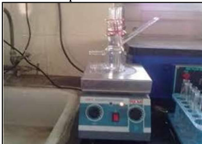
Fig no. 1 Franz diffusion cell to measure in-vitro drug permeation from buccal patch
