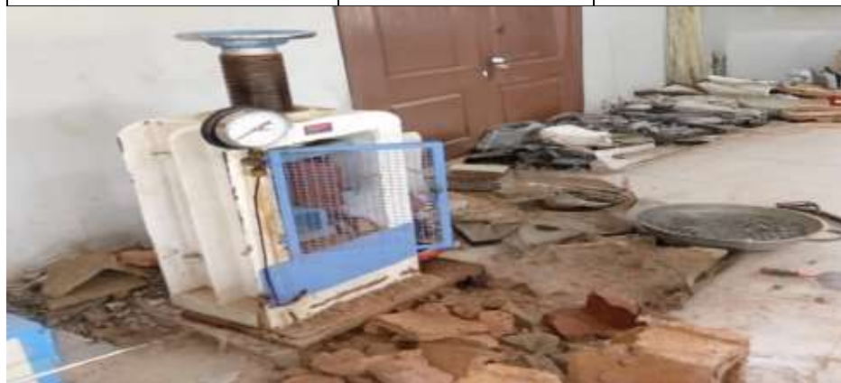
Plate 1: Crushing of the block samples using a compression machine
