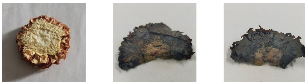
(a) Uncarbonized Corn Cobs (b) Corn Cob Carbonized at 250°C (c) Corn Cob Carbonized at 300°C
