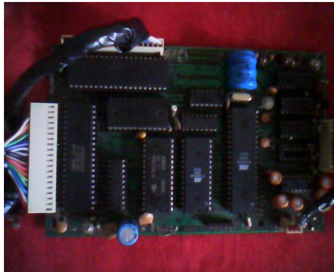
Figure 2: Fabricated Data Acquisition System
