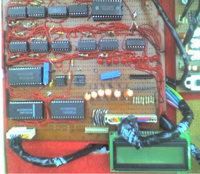
Figure 1: Fabricated Real Time Electrical Impedance Measuring System
