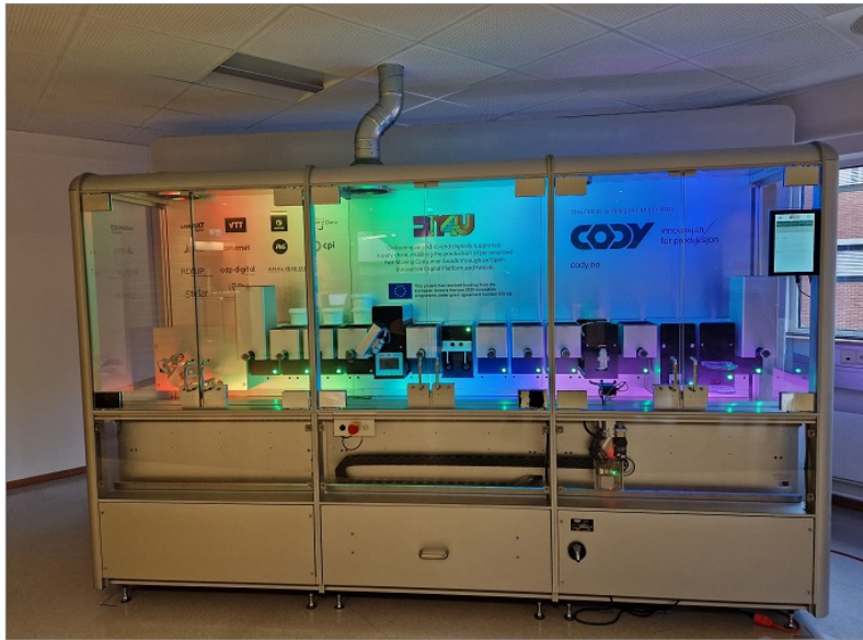
Figure 5: Modular manufacturing unit for personalized powder detergent Source: SINTEF (2019)
