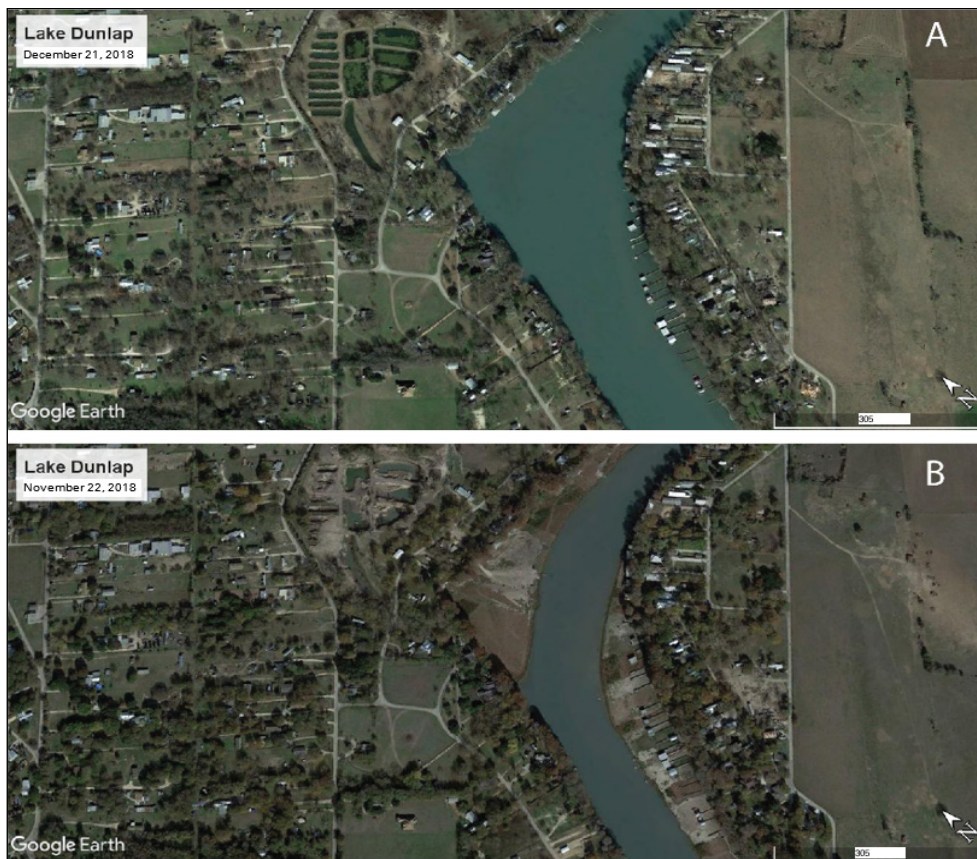
Figure 4. Zoomed lake comparison. Map depicting Lake Dunlap, Texas at its final bend before the dam. Version A shows imagery from 2018, before the dam failed ( Google Earth, n.d.-c ). Version B shows imagery from 2019, after the dam failed ( Google Earth, n.d.-d ).
