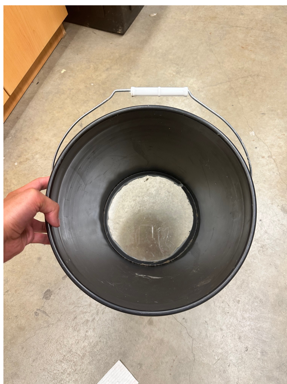
Figure 1, one of the clear-bottom buckets used to survey the Mussels.
