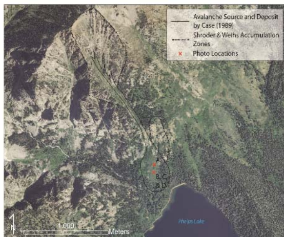
Figure 6. Planimetric view of Death Canyon avalanche source and deposit using NAIP aerial photo (2009). Avalanche polygon delineated by Case (1989) (solid line) was modified in this study (dashed line). Adjacent photos are located on map with red X's.
