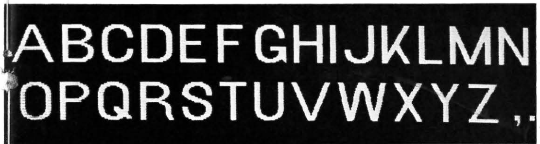
Figure 11. Video image of intermediate stage of Vidifont character. Curves are still flat-sided.
