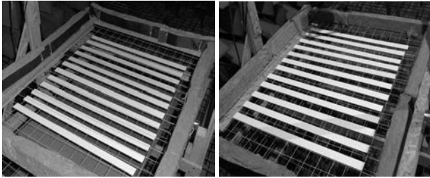
Fig. 4. Studied reflecting structure ( \mu = 0.6 , \varepsilon = 70 ) positioned over the reflecting plate simulating the ceiling and without this plate.
