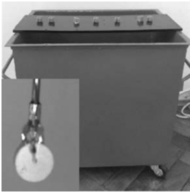
Fig. 1. View of the transformer tank and the transducer applied in the experiments.
