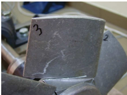
Fig. 8. Simulation of crack at blade no 3.
