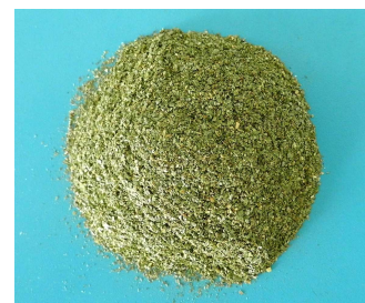
Fig. 1. Bamboo chips prepared for PU foam composites.
