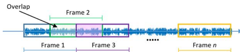
Fig. 4. Windowing is applied to minimize the discontinuities at the edge of each frame.
