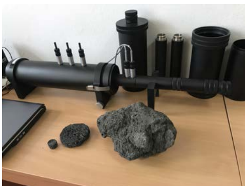
Fig. 10. Measuring stand with lava rock samples.
