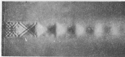
Fig. 8. Choked gas discharge from a disk ( n = 19 , \eta = 0.5 ) for various supply pressures
