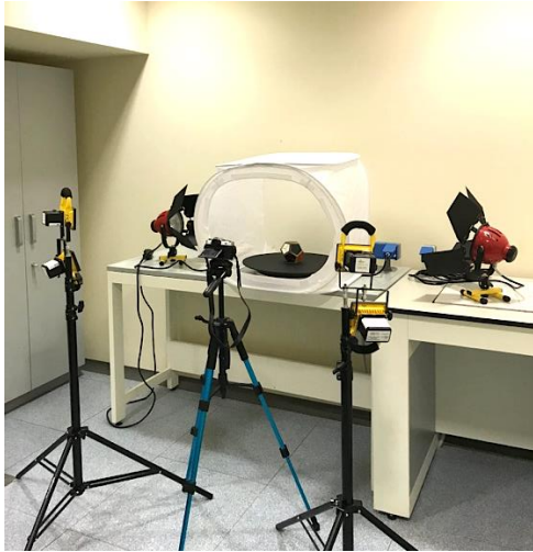
Figure 3. Photogrammetry system for multispectral images acquisitions.
