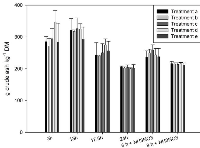
Fig. 1. Crude ash concentrations in different NaOH treated samples following increasing ashing times at  $550 \text{ }^{\circ}\text{C}$  (a–e, all  $120 \text{ g NaOH kg}^{-1}$ ; a:  $450 \text{ g DM kg}^{-1}$ , 2 d storage; b:  $600 \text{ g DM kg}^{-1}$ , 2 d; c:  $600 \text{ g DM kg}^{-1}$ , 7 d; d: like a [other batch]; e:  $450 \text{ g DM kg}^{-1}$ , 7 d). Error bars show the standard deviation.
