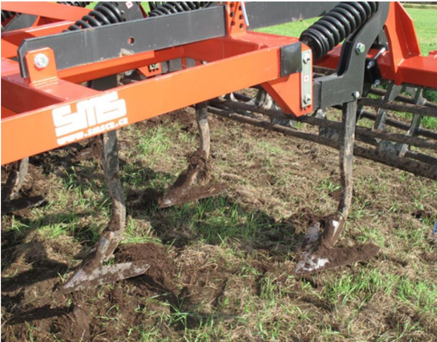
Suppl. Fig. 8. Tined cultivator with goosefoot blades was used in experiment 2 in the second year.
