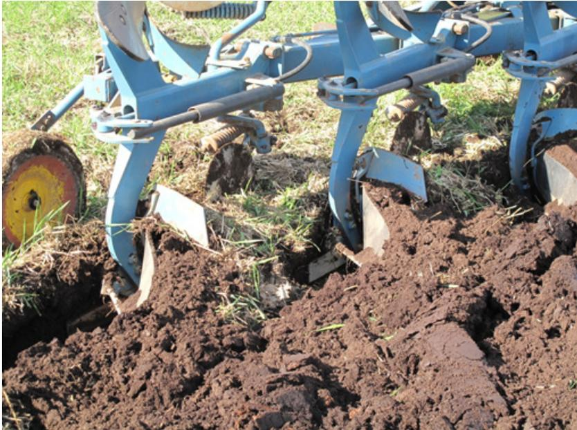
Suppl. Fig. 4. Trashboards installed on plough (above the mouldboards). This plough was used in experiment 1 and 2.
