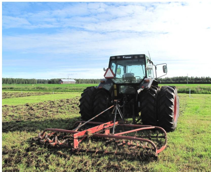
Suppl. Fig. 6. Rotary spade harrow which was used in experiment 1 in the second year and in experiment 2 in both years.
