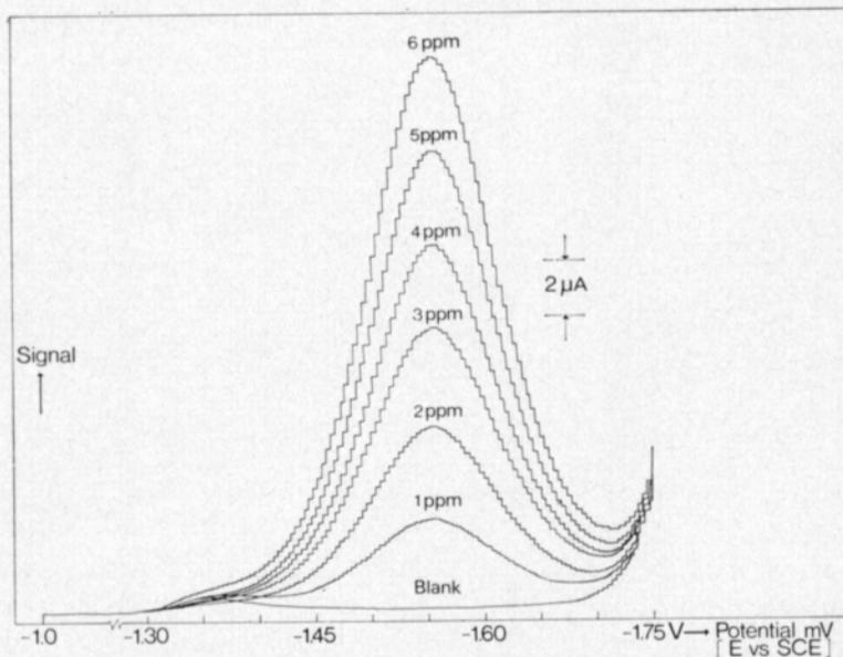
Fig. 1. Differential pulse polarogram of bromate ion in 1 M  $\text{NH}_4\text{Cl}/\text{NH}_4\text{OH}$  buffer  $[\text{Br(V)}] = 1-6$  ppm. Scan rate = 2 mV/sec. Drop time = 2 sec.
