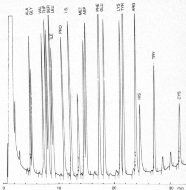
detector and injection block was 250°. The flow rate of the carrier N<sub>2</sub> was 30 ml/min.
