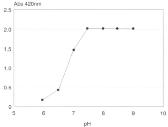
Fig. 5. pH profile of fibre-entrapped  $\beta$ -galactosidase with ONPG as substrate.
