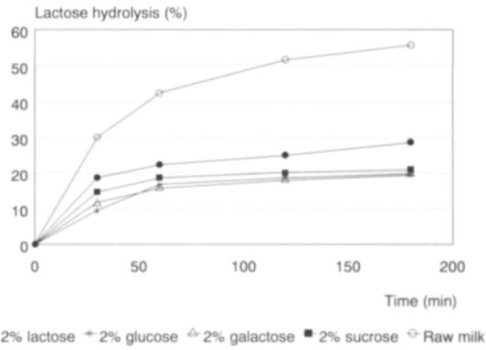
Fig. 3. Hydrolysis of lactose at 55°C in milk with added sugars. 8 ONPG units of enzyme activity were added per ml of milk.
