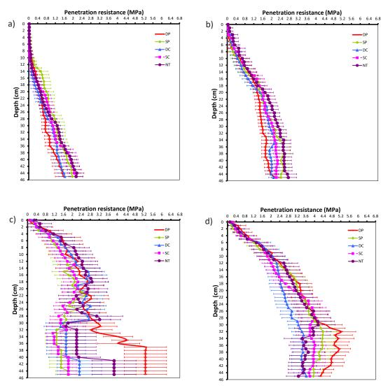
Fig. 3. Soil penetration resistance at different stages of experiment in 2018: a) before pre-sowing tillage in spring; b) after faba bean sowing; c) beginning of faba bean flowering; d) after harvesting. DP = deep ploughing, SP = shallow ploughing, DC = deep cultivation, SC = shallow cultivation, NT = no-tillage (direct drilling).
