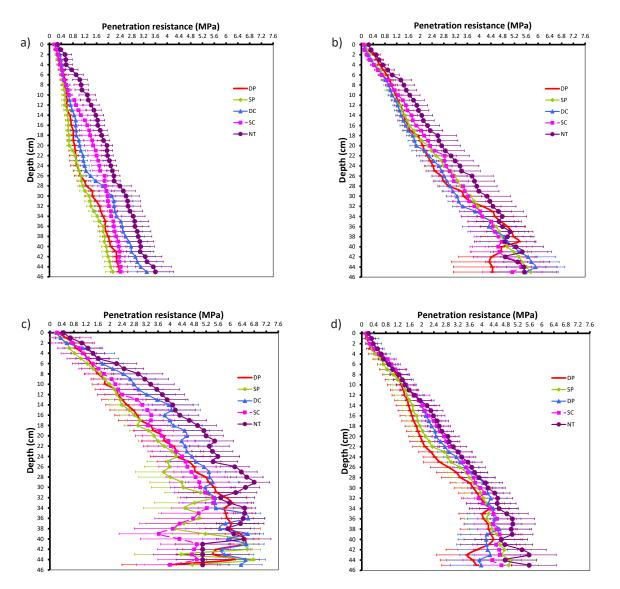
Fig. 2. Soil penetration resistance at different stages of experiment in 2017: a) before pre-sowing tillage in spring; b) after faba bean sowing; c) beginning of faba bean flowering; d) after harvesting. DP = deep ploughing, SP = shallow ploughing, DC = deep cultivation, SC = shallow cultivation, NT = no-tillage (direct drilling). Horizontal bars mean standard deviation.
