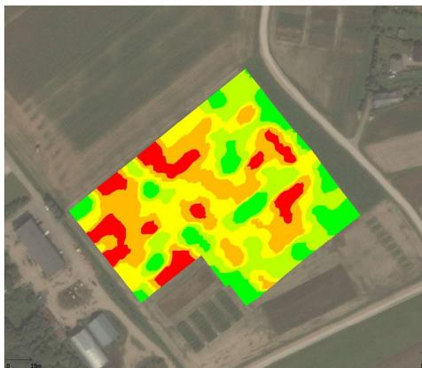
Fig. 3. Experimental site mapping with Veris 3150 MSP
