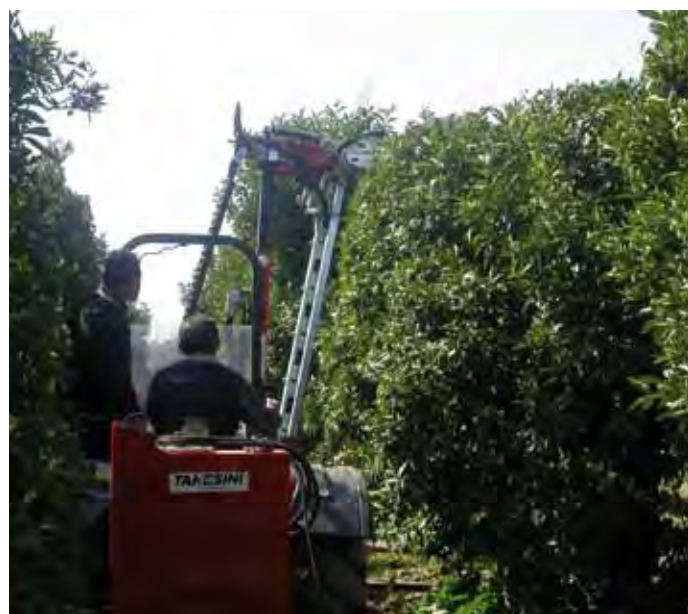
Fig. 8 - Mechanical hedging and topping done at the same time.
