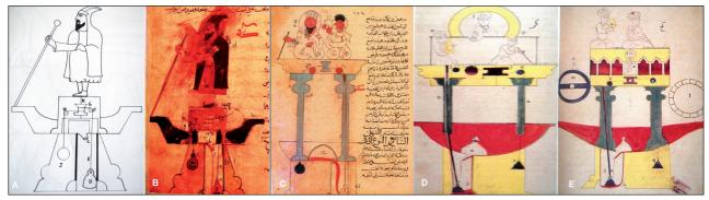
has been drained into the tank, the float rises and the "G" reel spins. In accordance with the spinning of the reel, the monk and its rod spin in a way that shows the amount of blood taken. The rod in the hand of the monk reaches the first sign once 1 dirham (dirham = 3.207 gr) of blood has been collected in the tank (5).
