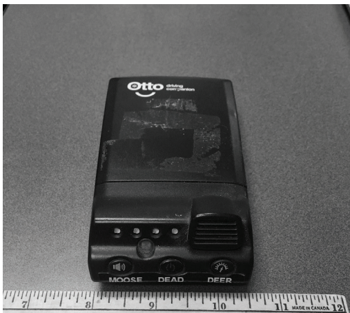
Fig. 1. The Otto® Wildlife GPS device used for capturing location data for live and dead deer/moose. The unit is powered by two AA batteries or can be plugged into the vehicle’s accessory receptacle.
