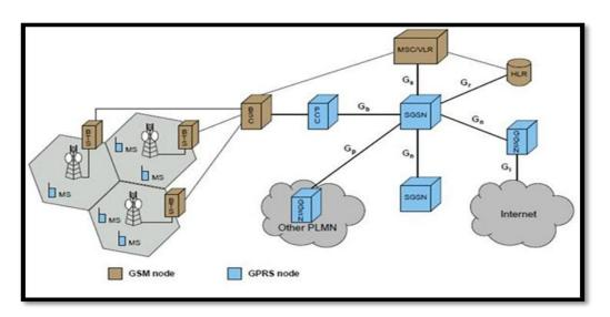
Fig. 1.GPRS Network Architecture [5].
