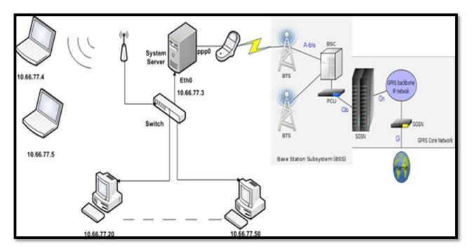
Fig. 2.Actual Implemented and Tested Network.
