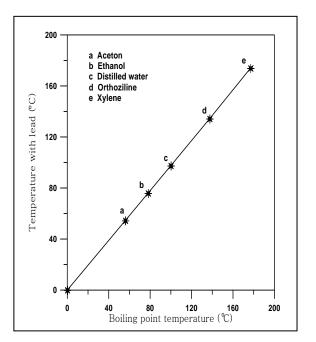
Fig. 11. b. Thermocouple Calibration Results.
