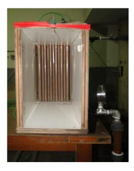
Fig. 6. Plain Tube Heat Exchanger.
