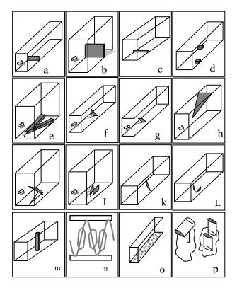
Fig. 2. Triangle and Rectangle Wings and Winglets.
