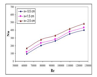
Fig. 16. Experimental Variation of Nusselt Number with Reynolds Number at Square Vortex Generators.
