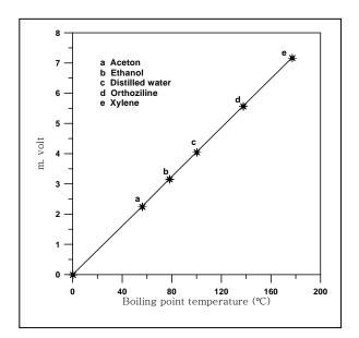
Fig. 11. a. Thermocouple Calibration Results.
