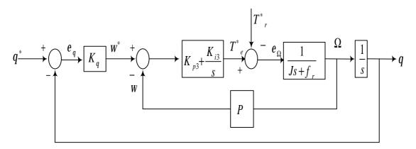
Fig. 1.Block Diagram of Position Regulation.
