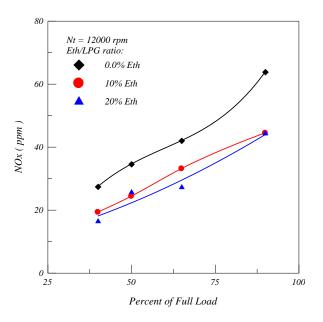
Fig. 5. Effect of Engine Loading on No<sub>x</sub> Emission.
