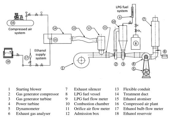
Fig. 1. Experimental Set-Up Showing the Spraying System Attached To the Gas Turbine.
