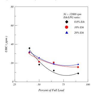
Fig. 7. Effect of Engine Loading on UHC Emission.
