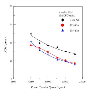
Fig. 2. Effect of Power Turbine Speed on  $No_x$  Emission.
