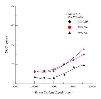
Fig. 4. Effect of Power Turbine Speed on UHC Emission.
