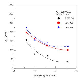
Fig. 6. Effect of Engine Loading on CO Emission.
