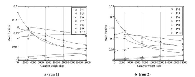
Fig. 7. Comparison between actual and simulated Paraffins composition (symbols actual, lines predicted).
