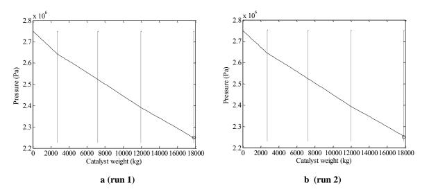
Fig. 5.Comparison between Actual and Simulated Pressure Drop (symbols actual ,lines predicted)
