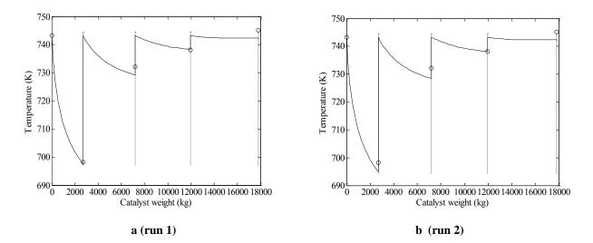
Fig. 4. Comparison between actual and simulated temperature profile (symbols actual, lines predicted).
