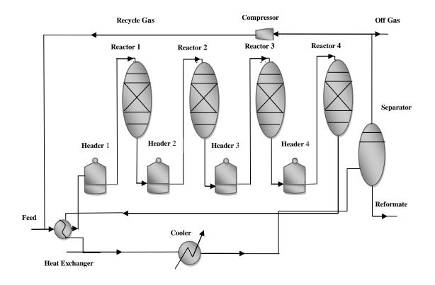
Fig. 1. Process flow of four reactors naphtha reforming process.
