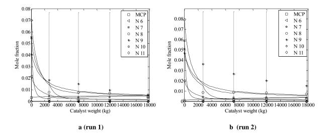
Fig. 8. Comparison between actual and simulated naphthenes composition (symbols actual, lines predicted).
