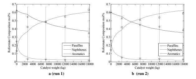
Fig. 6. Comparison between actual and simulated total Paraffins, naphthenes, and aromatics in reforming process (symbols actual ,lines predicted).
