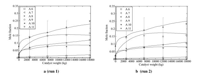
Fig. 9. Comparison between actual and simulated aromatics composition (symbols actual ,lines predicted).
