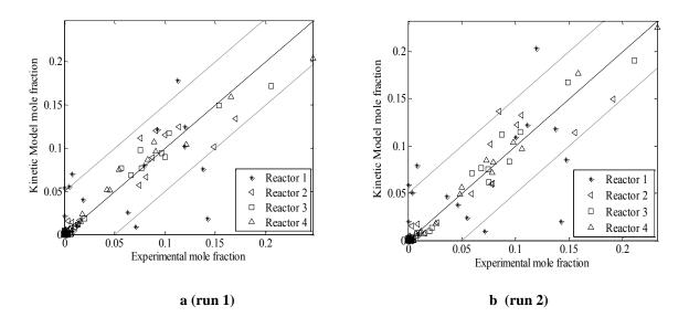
Fig. 3. Comparison between actual and simulated reformate compositions (symbols actual ,lines predicted).
