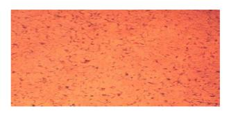
Fig.1. the microstructure of surface of low carbon steel specimen before it was buried in different media (200X).
