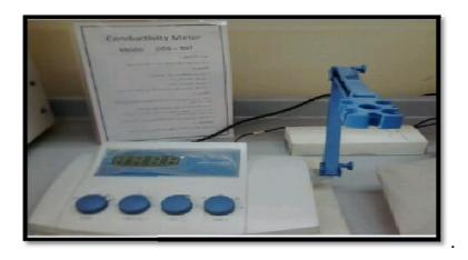
${\bf Fig. 3.\ Digital\ electrical\ conductivity\ meter.}$
